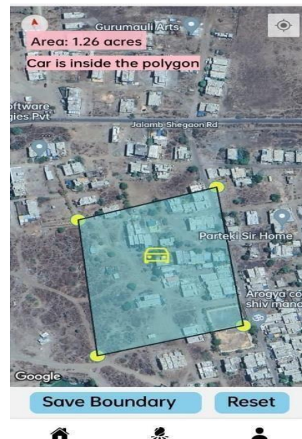
Fig3: Interface for tracking car location in Geofence
